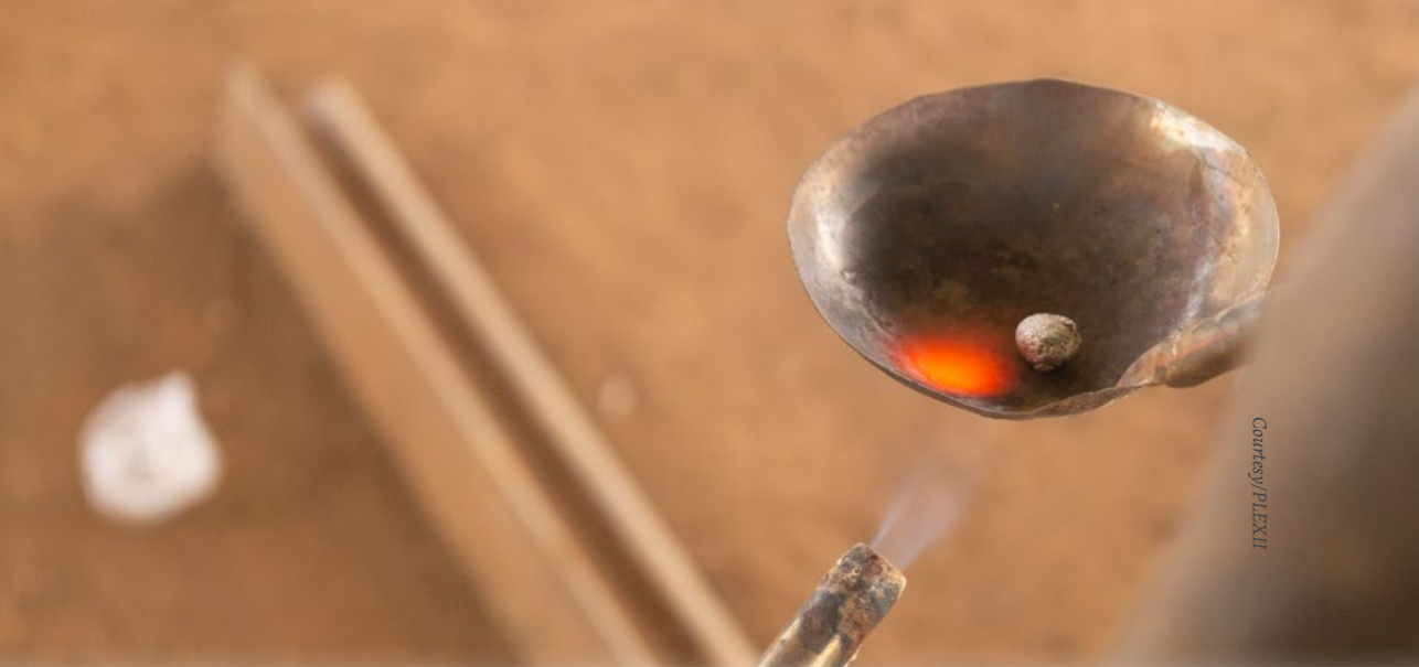
A photo showing burning of mercury and gold ore amalgam.
