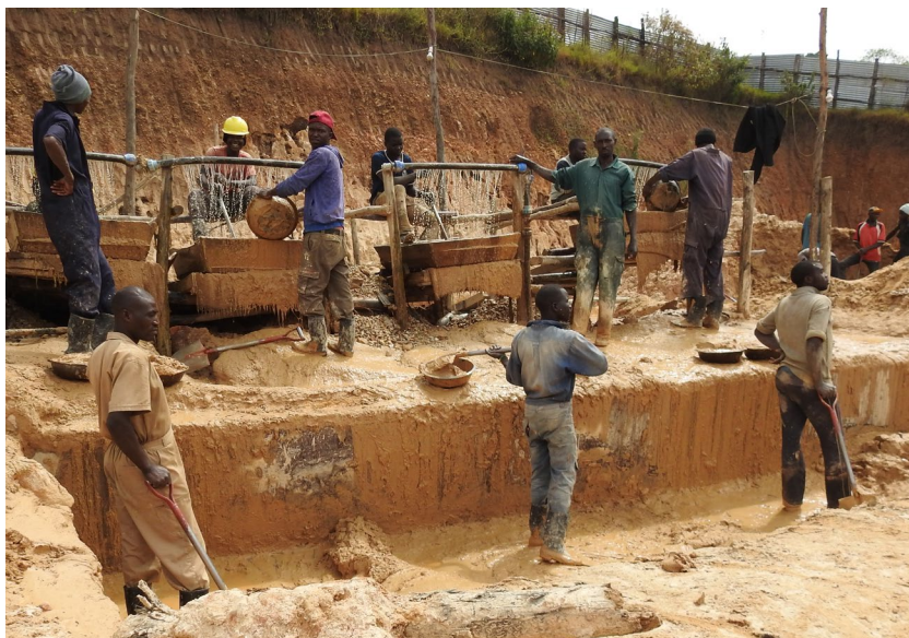
Gold miners at Katenga mining site in Buhweju washing gold ore using sluice boxes (PLEXII, 2018)
