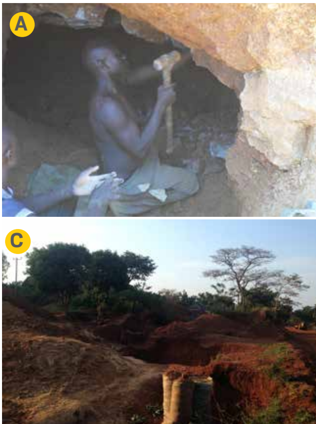
Figure 11: A: Miners working in groups breaking a rock from a quartz vein believed to be having gold at Nakudi mine site; B: Quartz vein/reef that has been extracted consisting of sulphide mineralisation and box work structures containing gold; C: Ore material from the Tiira pit packed in sacks ready for transporting to the milling site; D: Panning at the Tiira river; E: Drying and milling site for the rocks; F: A miner holding a mercury amalgam on bare hands which can be a health risk.
