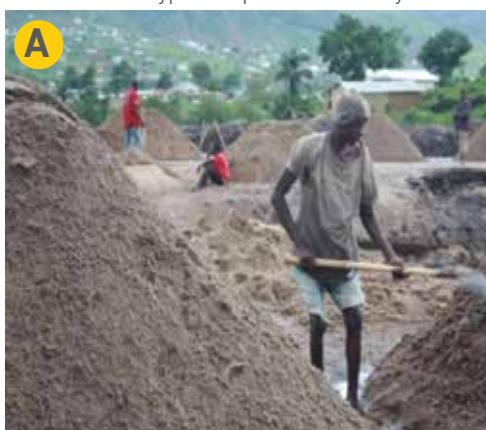
Figure 20: A- ASM digging sand using hoes and shovels in Lwera; B: Sand excavation and loading on trucks using an excavator at Katosi.
