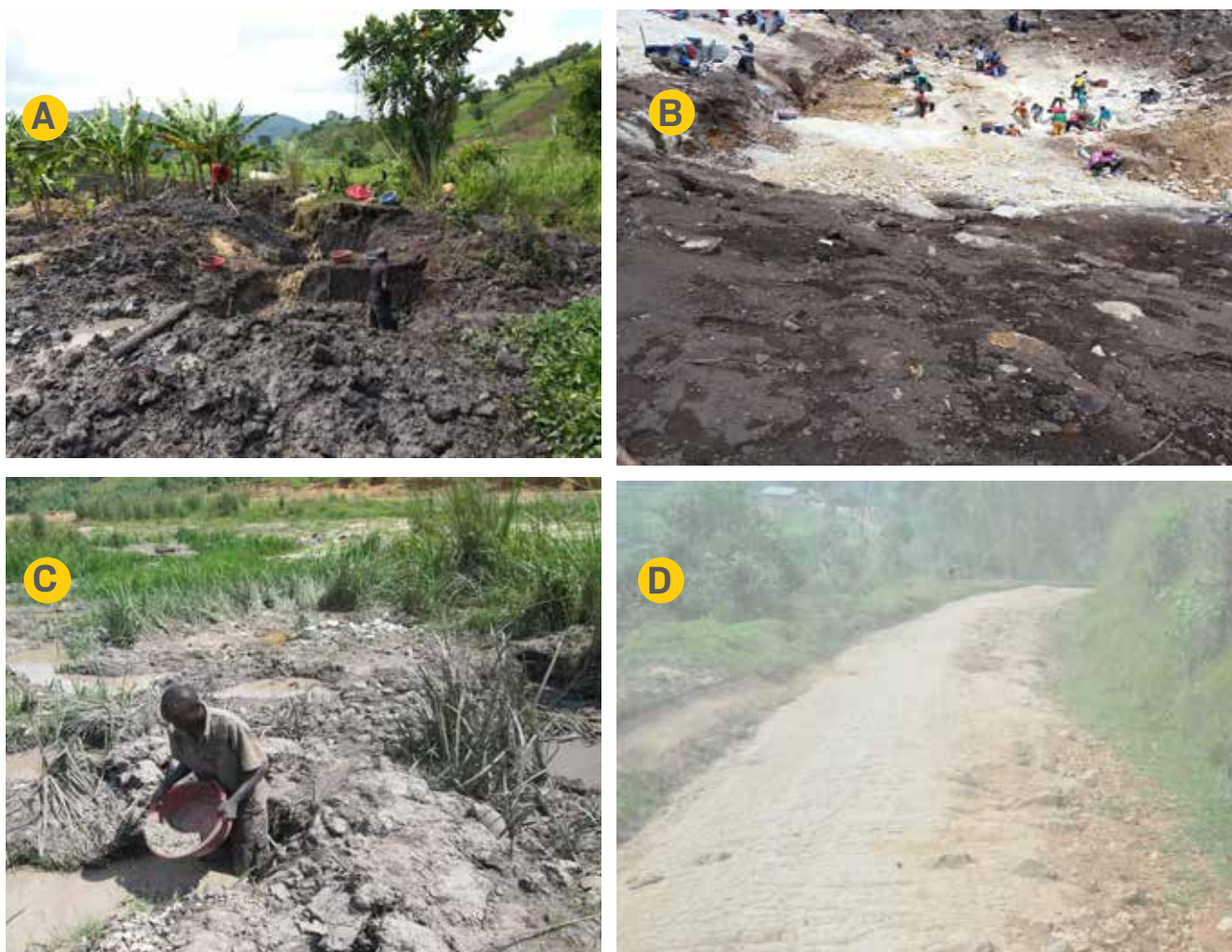
Figure 13- A: Miners digging pits for gold in swampy areas of Buhweju; B: Young energetic men and women miners excavating gravel from one of the open pits and ferrying the ore using basins to the surface; C: A miner panning for gold from sand using a basin in a swamp; D: The poor road network to the mining site in Buhweju District.
