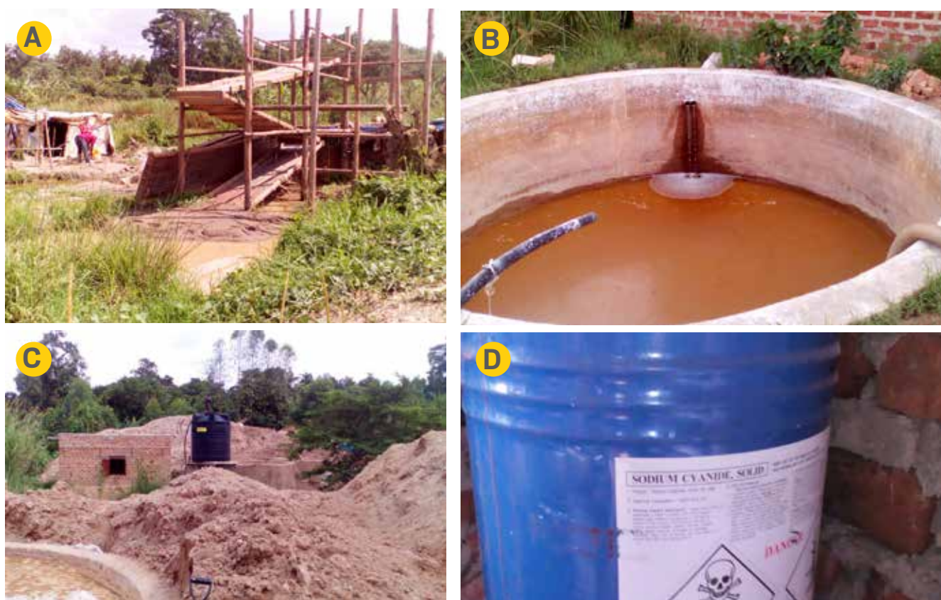
Figure 8: A: The Zig-Zag sluice box; B and C Barren leaching tank for mixing chemicals; D Cyanide drum containing the cyanide imported and used;
