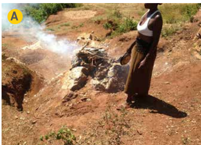
Figure: 26- A miner burning firewood on the rock surface in Tororo limestone quarry; B: Male miners breaking large rocks.
