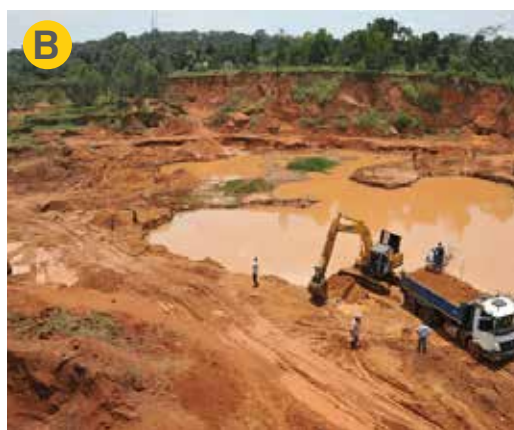
Figure 20: A- ASM digging sand using hoes and shovels in Lwera; B: Sand excavation and loading on trucks using an excavator at Katosi.
