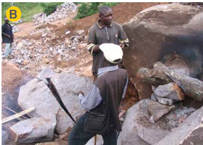
Figure: 26- A miner burning firewood on the rock surface in Tororo limestone quarry; B: Male miners breaking large rocks.
